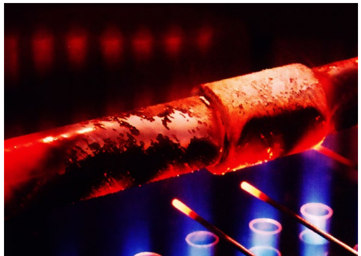
Fire endurance testing of Bondstrand fiberglass pipe and fitting
